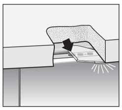
When the dishwasher is built-in, the left hand side of the reflector panel must be sited above the in-operation light in the dishwasher control panel.
